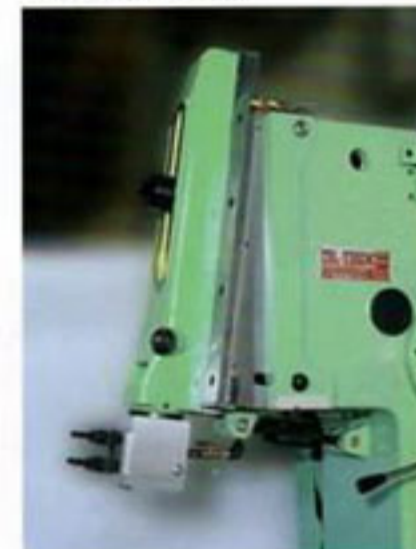
▲ 鉋頭可傾斜 Inclinable Ram for taper hole
